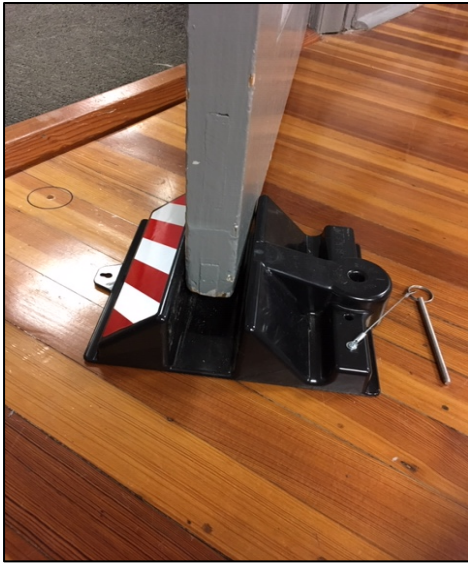
1. Slide Bearacademy device onto door.
