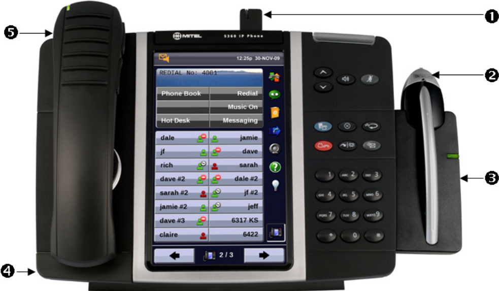
DECT Cordless Module and Accessories on a 5360 IP Phone
